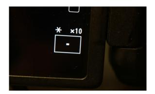
6. Focus your image using the focus ring, and then press the shutter release to begin capturing images!
