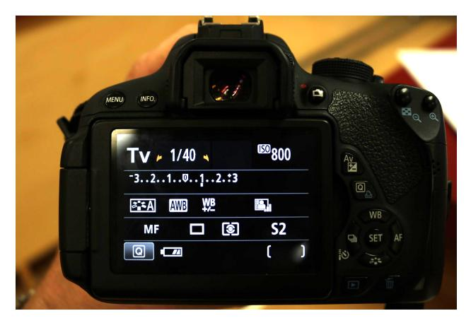
To adjust any of the settings, press the "Q" button to the right of the screen. This will allow you to scroll around the settings.
